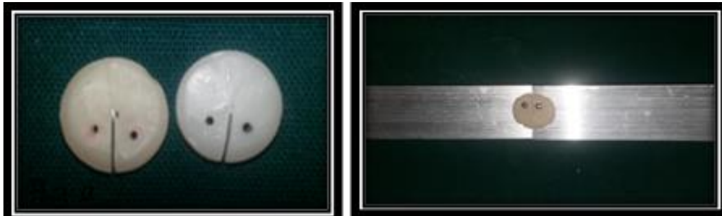
Fig: 2 (a). Pre crack was made on the samples using diamond disk; (b) Sample attached to jig
