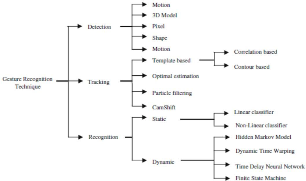
Fig. 5: Vision based hand gesture recognizing techniques.
