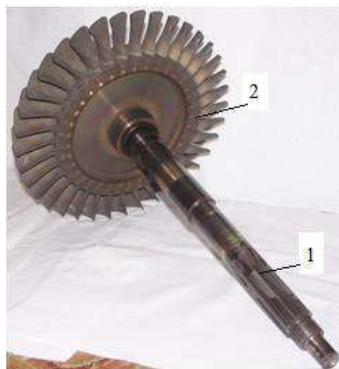
Fig. 3.2: Rotor shaft of the turbocharger with a disk: 1 - shaft; 2 - blade with blades.
