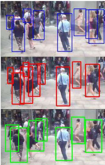
Fig. 3: shows the results of using pedestrian detection methods (from top to bottom): SSD, YOLO, HOG+SVM.
