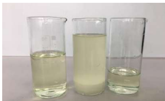
Fig. 3: Left to right: source gasoline; emulsion with 10.6% water in gasoline; gasoline, purified from water absorbent.
