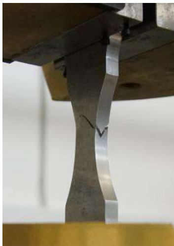
Fig. 6: View and results of fatigue tests on specimens made of 1915T aluminium alloy
