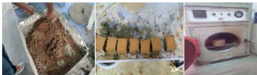
Fig. 2: Mixing, Casting and Oven Curing
