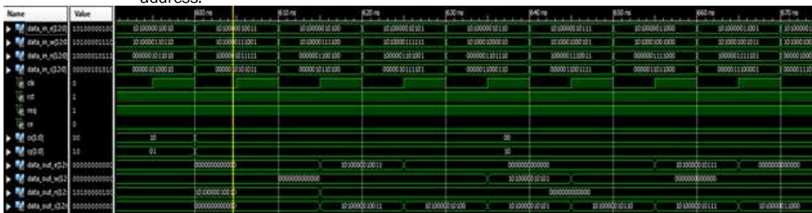
Fig. 13: Simulation result of the proposed NoC transferring data at South Port.
