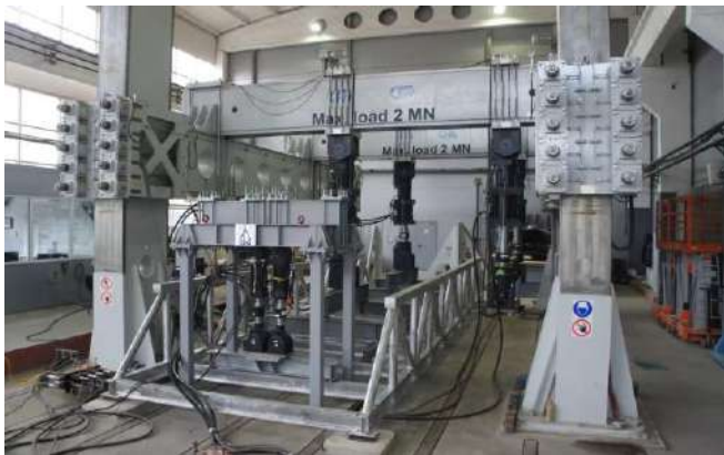
Fig. 7: View of the test on walking bridge made of 1915T aluminium alloy
