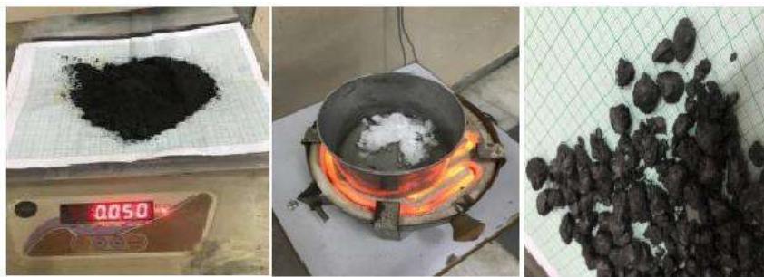
Fig. 1: PCM Preparation paraffin wax and graphite powder
