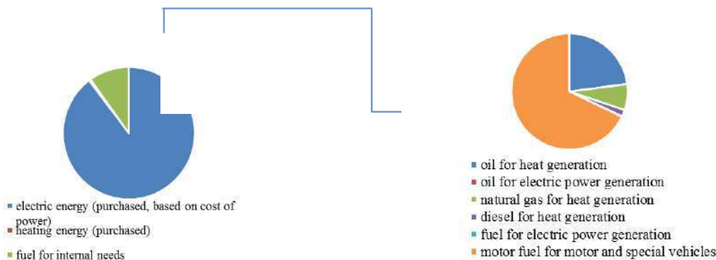
Fig. 4: Structure of energy consumption at a midstream oil enterprise in the reporting year, % (developed by the authors based on the enterprise's data)
