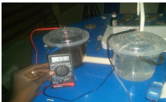
Fig. 1: A double chambered MFC consisting of an anaerobic chamber (anode; left) and aerobic chamber (cathode; right) connected by pvc pipe salt bridge.
