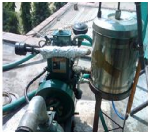
Fig.1 Heating arrangement for JO
