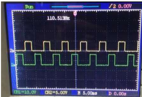
Fig.4.29: Switching pulse for M1,M3
