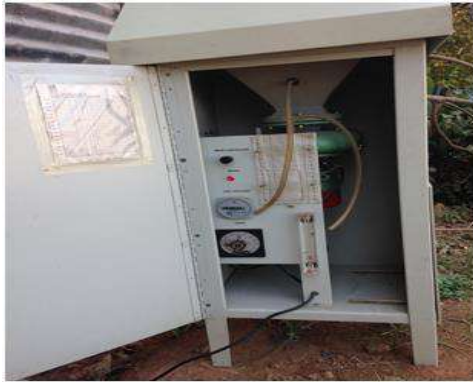
Fig. 1: Inside view of high volume air sampler
