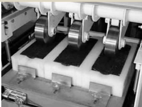
Fig. 3: Experimental setup for PT fatigue test method.
