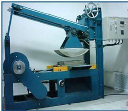
Fig: 2. Roller compactor machine
