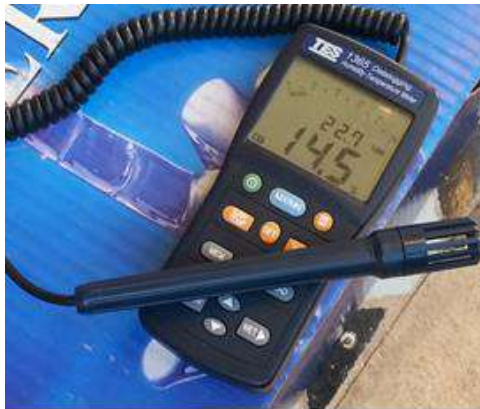
Fig: 7. the applied instrument to measure the temperature and humidity
