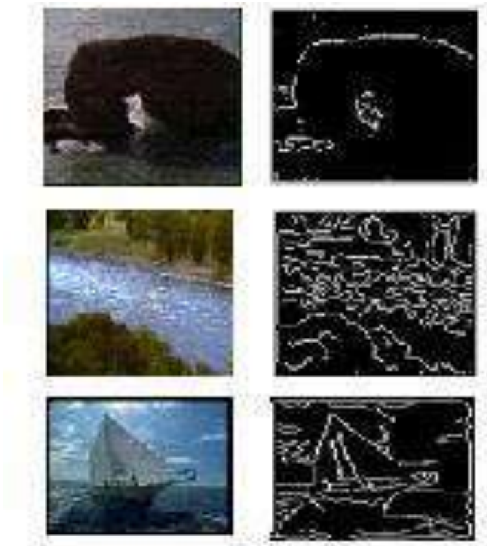
Fig: 3. Input Image is on the Left, Gradient Images on the Right
