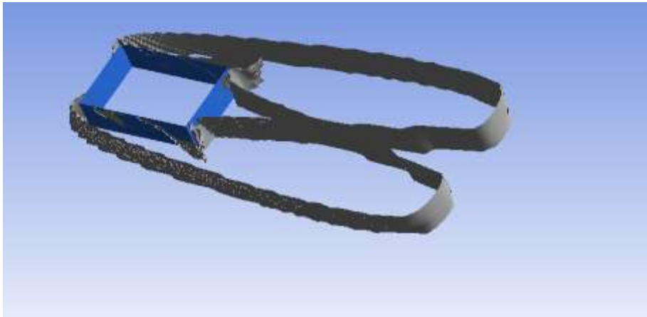
Fig: 3. Eddy around square column at re=50000
