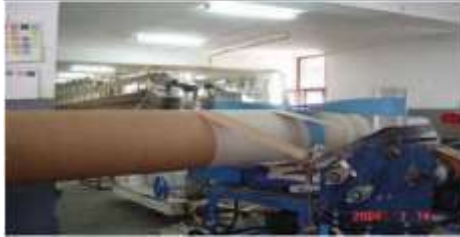
Fig. 1: The machine which turns paper sheets into paper pipes.
