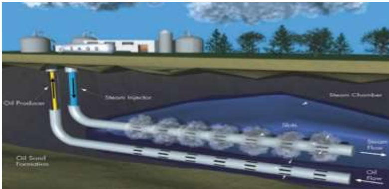
Fig. 13: SAGD process ( Source : Canadian Center for Energy Information)
