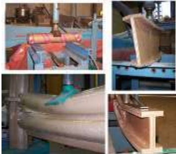
Fig. 2: Examining mechanical strength of structural paper components.
