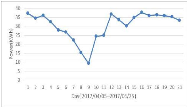
a. Daily production diagram of the photovoltaic system in a 21-day period
