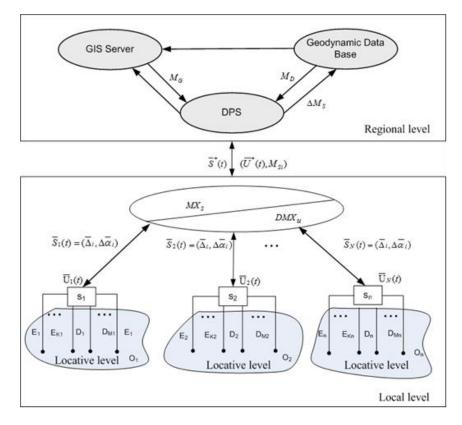
Fig. 1: The generalized scheme of the information processing of geo ecological monitoring data.
