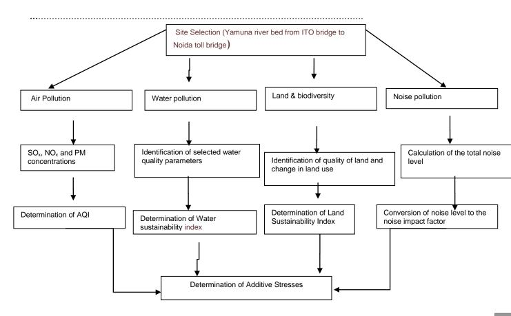
Fig.4: Methodology for determination of additive stresses
