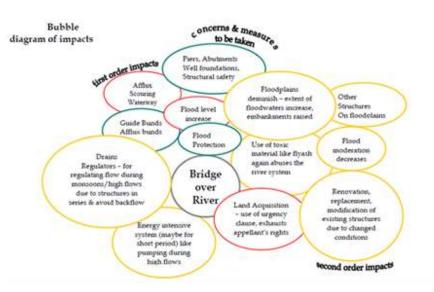
Fig: 3. Conceptual Diagram showing the effect of structures on the river [1]
