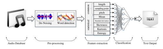
Fig. 1: Architecture of Proposed ASR system
