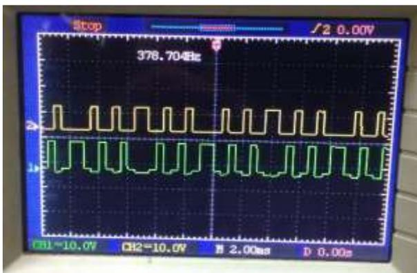
Fig.4.30: Switching pulse for M5, M7
