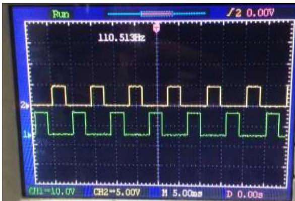
Fig.4.29: Switching pulse for M1,M3
