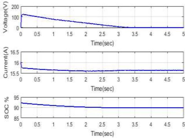
Fig.13: Battery states of charge in case 2.
