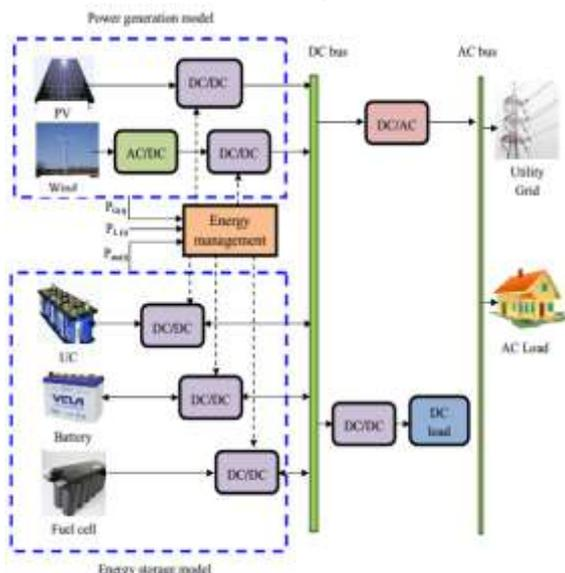
Fig. 1: Proposed schematic diagram of the REMS
