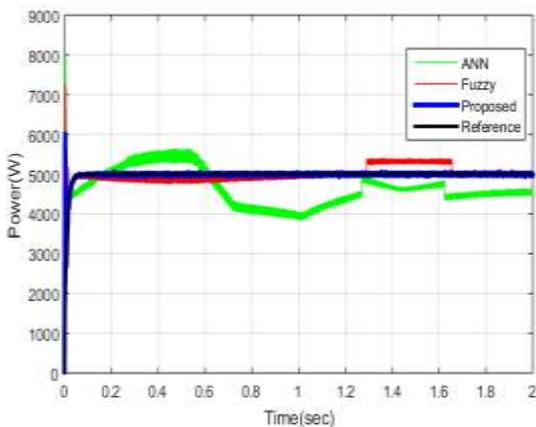
Fig.14: The comparison investigation of the generated power with dissimilar methods
