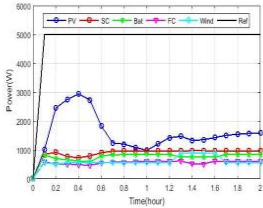
Fig. 6: Power produced from the existing sources SC, Battery, FC, PV and WT in case 1.
