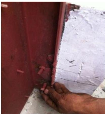
Fig. 6(a): Bending of the bolts.
