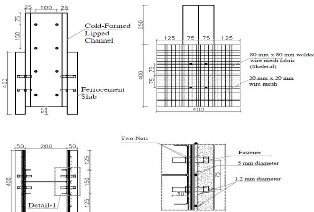
**Fig. 1:** Layout for push-out test specimen.
