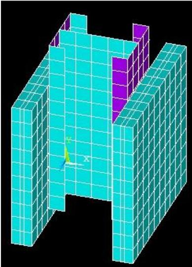
Fig. 5: Typical composite beam FE mesh .
