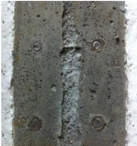
Fig. 6(c): Failure in concrete around the bolts.
