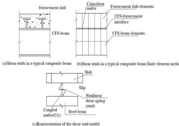
Fig. 4: Modelling of shear connectors.
