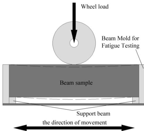
Fig. 4: Sample load for PT fatigue test method.
