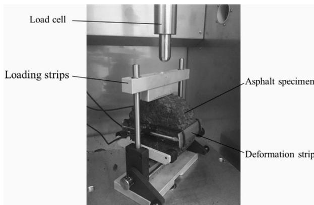
**Fig. 2:** Sample load for EN 12697–24 indirect tensile test.
