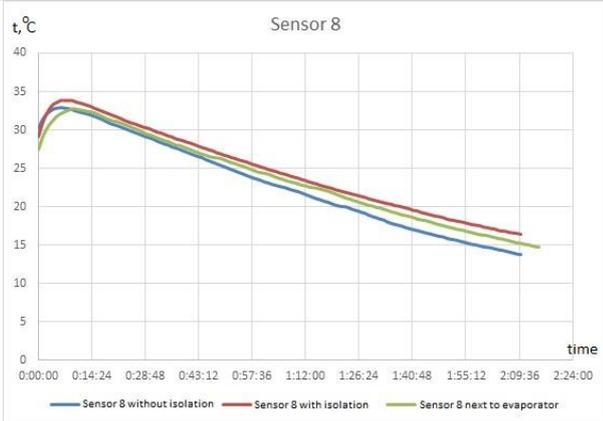
Fig.11: Graphs the surface temperature of the evaporator in embodiments 3.
