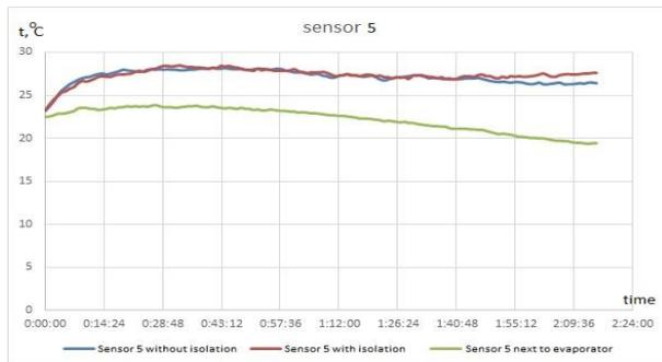
Fig.10: Temperature plots in the space between the evaporator and the compressor in embodiments 3.
