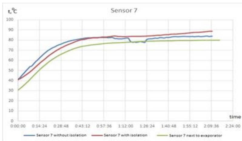
**Fig.8:** Temperature Charts compressor cap with 3 versions.
