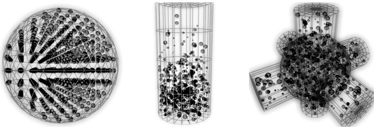
**Fig. 1:** Examples of initial particle distributions, left to right: simple cubic lattice of particles inside spherical boundary; 1D-normal, 2D-uniform distribution of particles inside cylinder; 3D-uniform distribution of particles inside complex CSG object.
