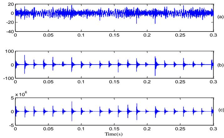
Fig. 3: (a) Raw signal (b) Third differentiation (c) twentieth differentiation.
