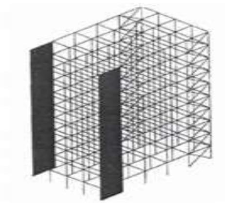
**Fig: 11 . third stage analysis - frame shear walls and steel bracings under the force of the earthquake(fwb1)**
