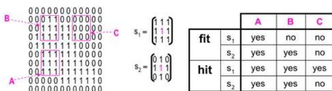
Fig. 6: Fitting and hitting of binary image with structuring elements s<sub>1</sub> and s<sub>2</sub>.
