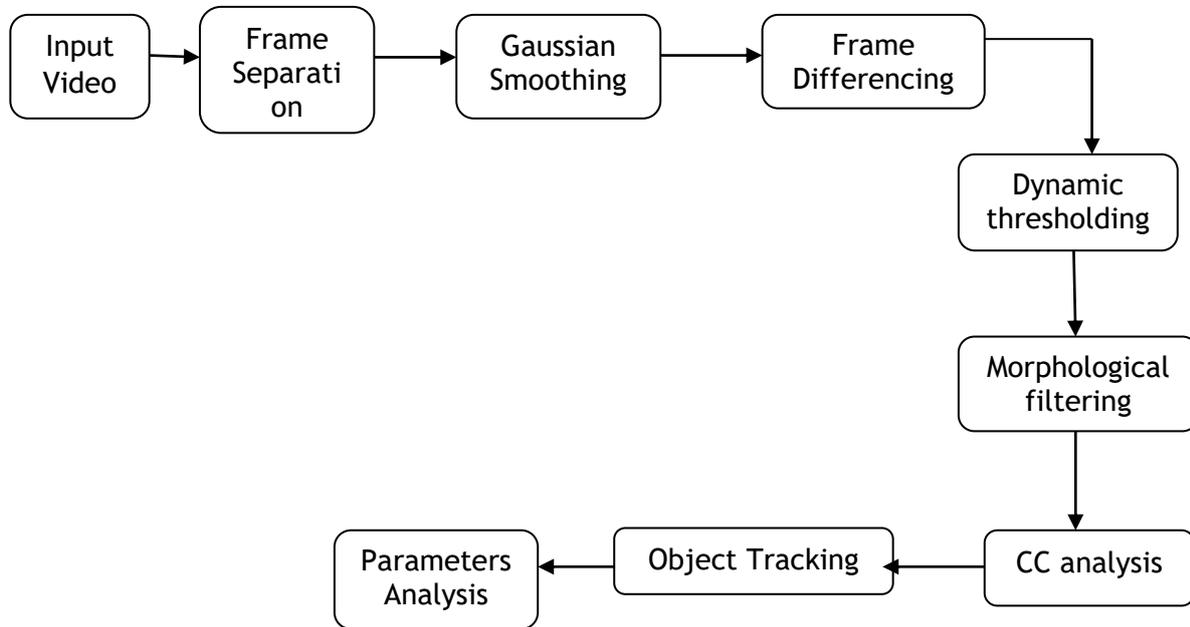
**Fig.1:** Block Diagram of Entire System
