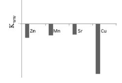
Fig. 2: Coefficient of concentration of ingredients of aqueous extract of solid pyrolysis product after ashing relative to TLV forwaste water in base 10 logarithmic scale.
