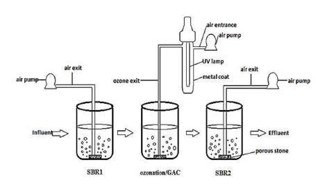
Fig .1: The schematic diagram of SBR1-O3/GAC-SBR2 was used in this study.
