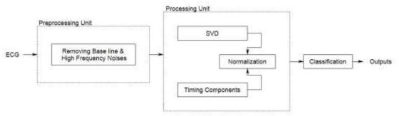
Fig.2 : Diagram of the proposed method for the diagnosis of cardiac arrhythm
