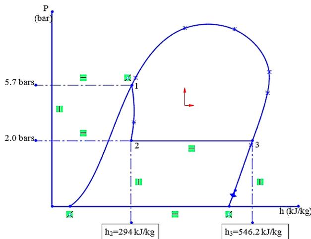
Fig. 3: The p-h diagram of refrigeration system.
