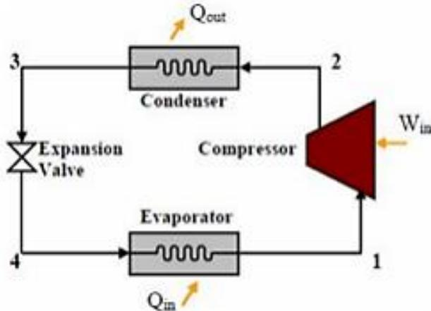
Fig. 1: Vapour compression refrigeration system cycle. [5]
