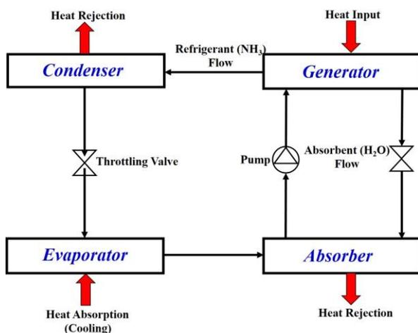
Fig. 1: Block diagram of NH<sub>3</sub>-H<sub>2</sub>O refrigeration system [10].
