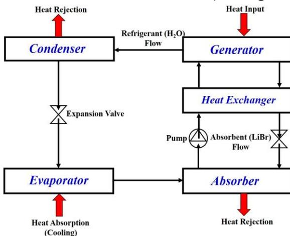
Fig. 2: Block diagram of  $\text{H}_2\text{O}$ -LiBr refrigeration system [24].
