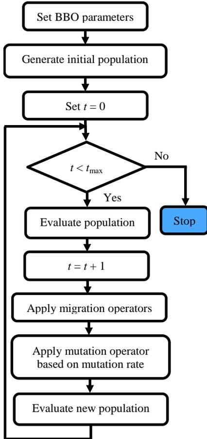
Fig. 3: Flowchart of the proposed optimization algorithm
