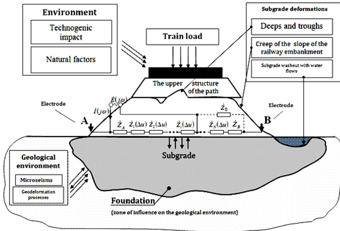
Fig. 2: The principle of application of seismo electric control of the subgrade of railway tracks
