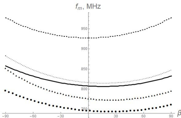
**Fig. 4:** Dependence of  $f_m$  on  $\beta$ . The solid line corresponds to  $r=1.0$  mm and the DBKP of the 1st order; the dotted line –  $r=2.0$  mm and the DBKP of the 1st order; circles –  $r=1.0$  mm and the DBKP of the 2nd order; triangles –  $r=2.0$  mm the DBKP of the 2nd order. The dashed line – the ordinary dipole with  $r=1.0$  mm.  $l = 7.5$  cm.
