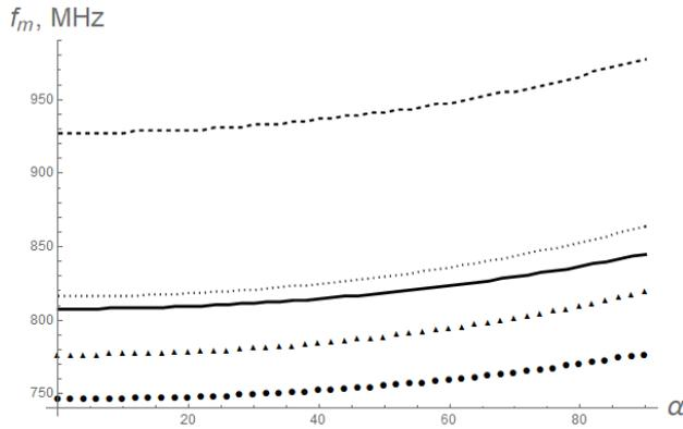
**Fig. 3:** Dependence of  $f_m$  on  $\alpha$ . The solid line corresponds to  $r=1.0$  mm and the DBKP of the 1st order; the dotted line –  $r=2.0$  mm and the DBKP of the 1st order; circles –  $r=1.0$  mm and the DBKP of the 2nd order; triangles –  $r=2.0$  mm the DBKP of the 2nd order. The dashed line – the ordinary dipole with  $r=1.0$  mm.  $l = 7.5$  cm.
