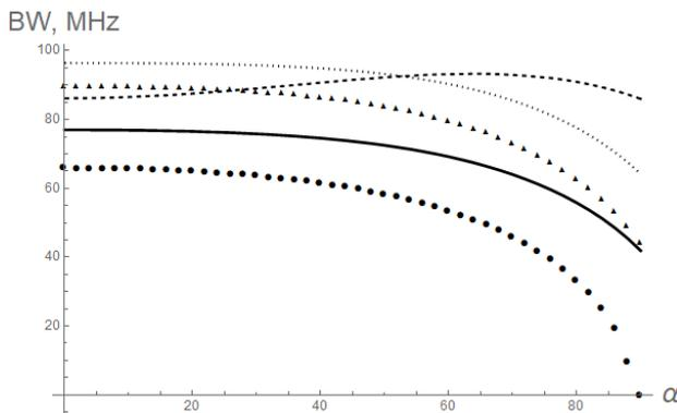
**Fig. 5:** Dependence of BW on the rotation angle  $\alpha$  of the arm around the  $y$ -axis relative to the normal dipole. The solid line corresponds to  $r=1.0$  mm and the DBKP of the 1st order; the dotted line –  $r=2.0$  mm and the DBKP of the 1st order; circles –  $r=1.0$  mm and the DBKP of the 2nd order; triangles –  $r=2.0$  mm and the DBKP of the 2nd order. The dashed line – the ordinary dipole with  $r=1.0$  mm.  $l = 7.5$  cm.
