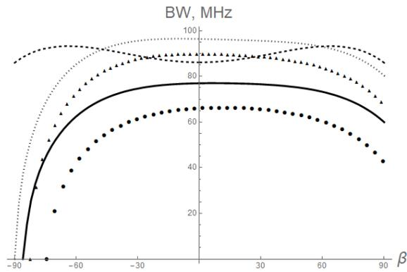
**Fig. 6:** Dependence of BW on the rotation angle  $\beta$  of the arm around the z-axis relative to the normal dipole. The solid line corresponds to  $r=1.0$  mm and the DBKP of the 1st order; the dotted line –  $r=2.0$  mm and the DBKP of the 1st order; circles –  $r=1.0$  mm and the DBKP of the 2nd order; triangles –  $r=2.0$  mm and the DBKP of the 2nd order. The dashed line – the ordinary dipole with  $r=1.0$  mm.  $l = 7.5$  cm.
