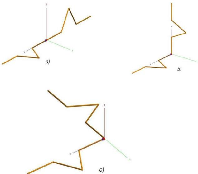
**Fig. 2:** Options for rotation of an arm around the axes: a) rotation around the  $x$ -axis (twisting); b) rotation around the  $y$ -axis; c) rotation around the  $z$ -axis.
