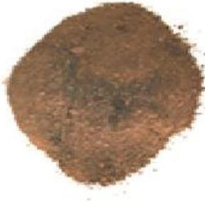
**Fig. 1:** Solid pyrolysis product after ashing.
