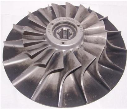
**Fig. 3.3:** The impeller of the compressor.
