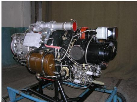
**Fig. 3.1:** General view of the turbo-generator unit TG-16M.
