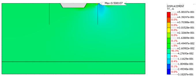
Fig. 12: Deformations from excavator and dump truck weight during the development of the fifth layer of soil.
