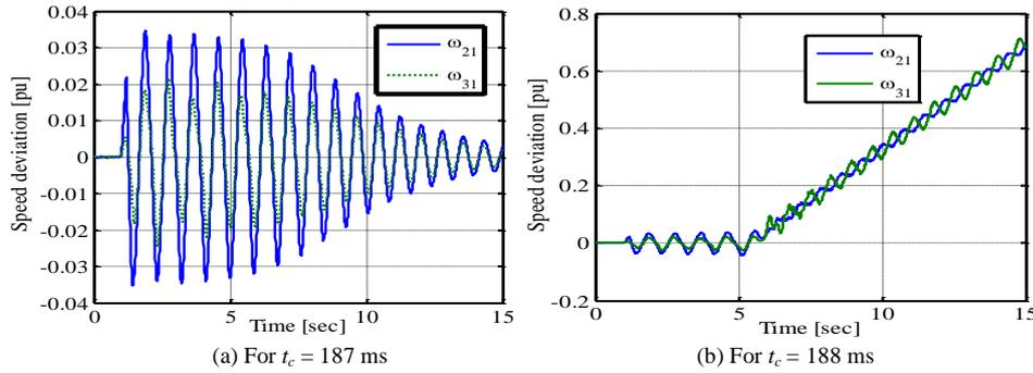
Fig. 1: Change in speed deviations for WSCC system
