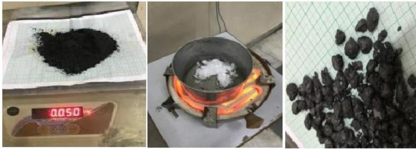
Fig. 1: PCM Preparation paraffin wax and graphite powder
