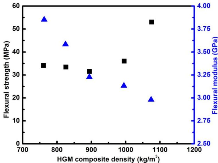
Fig. 6: Variation in flexural strength and modulus regarding the HGM composite density containing HGMs of 460 kg/m<sup>3</sup> density (Reconstructed from Reference [15]).
