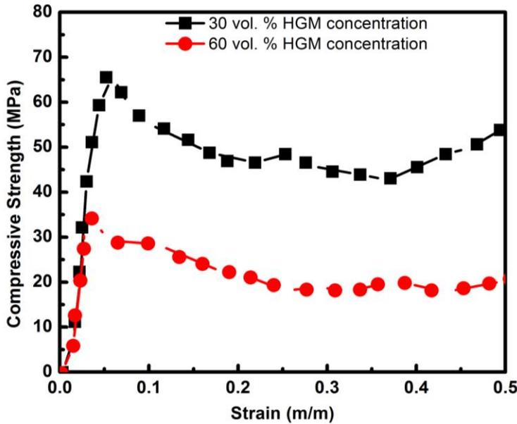
Fig. 1: Compressive stress-strain curve of epoxy matrix containing HGMs of 220 kg/m<sup>3</sup> in 60 and 30 vol% (Reconstructed from reference [13]).
