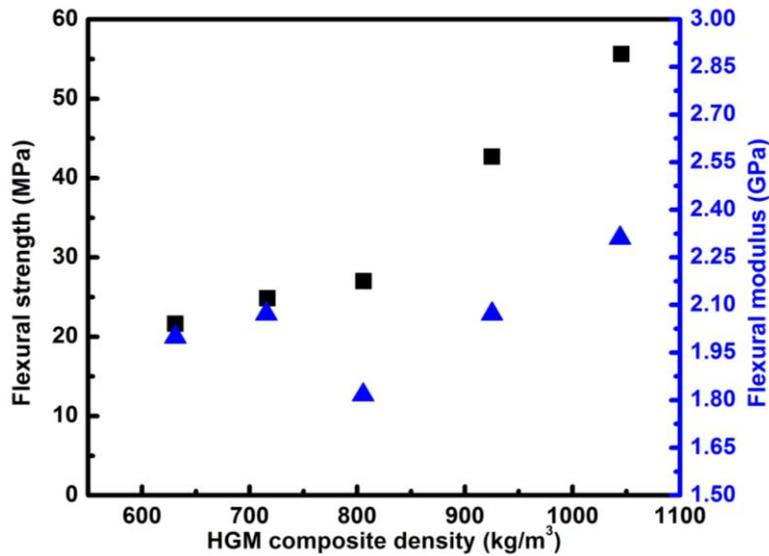
Fig. 5: Variation in flexural strength and modulus regarding the HGM composite density containing HGMs of 150 kg/m<sup>3</sup> density (Reconstructed from Reference [15]).
