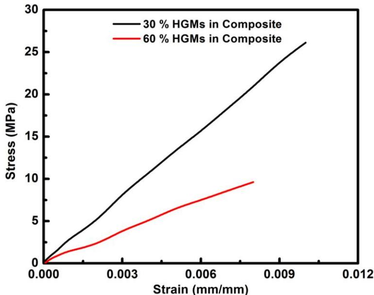
**Fig. 3:** Tensile stress-strain curves of HGM composites containing HGMs of 220 kg/m<sup>3</sup> density (Reconstructed from Reference [21]).
