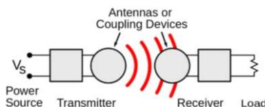
Fig. 1: An illustration of wireless power transfer
