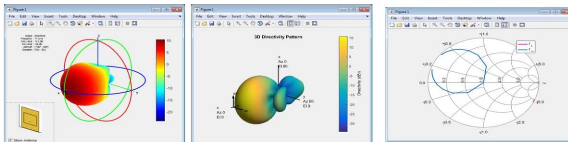
Fig. 4: Far field 3D radiation and directivity pattern for circular loop antenna.
