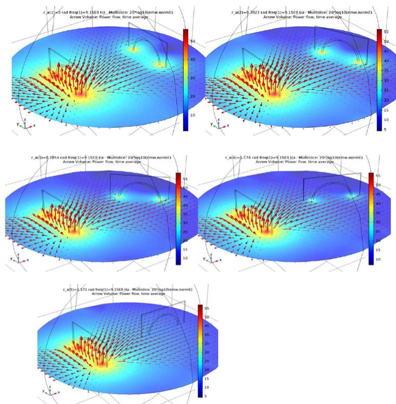
Fig. 5: Plot of E-field norm and power flow at  $z = 0$  while the receiving antenna is rotating from 0 to 90 degrees with a step of 22.5 degrees.
