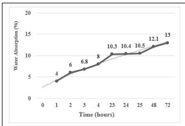
Fig. 2: Water absorption of Lightweight aggregates (*LECA*).
