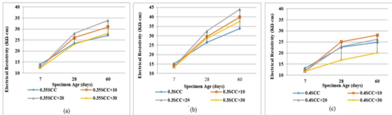
Fig. 9: Electrical resistivity of concrete specimens.
