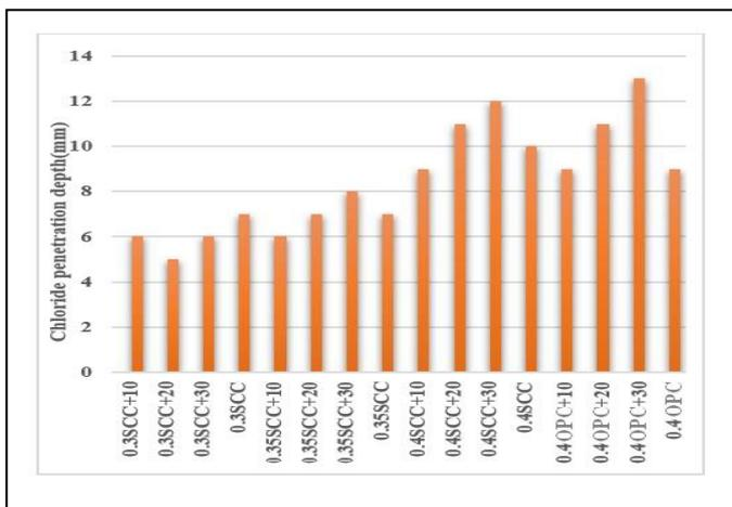
Fig. 8: Chloride penetration depth after 28 days.
