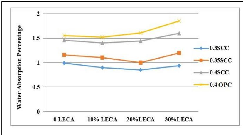
Fig. 7: The water absorption of concrete specimens.
