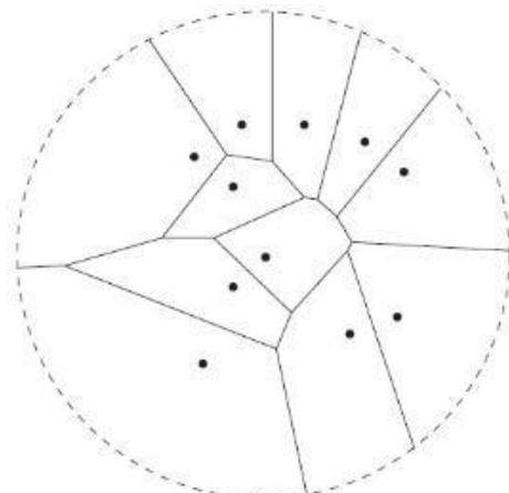
**Fig. 3:** A Voronoi diagram of 11 points in the Euclidean plane
