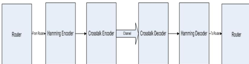
Fig. 5: Flow of the proposed Hybrid model
