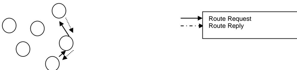
**Fig. 2:** Propagation of route request and route acknowledgement
