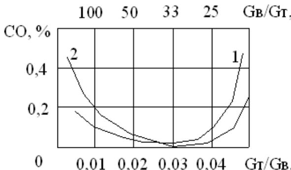
Fig. 2: Influence of mixture composition on CO emissions in direct injection diesel engines: 1 – supercharged diesel; 2 - diesel with free inlet.
