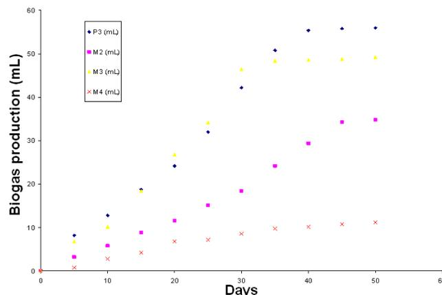
**Fig: 1. Cumulated biogas production at 50 days HRT**
