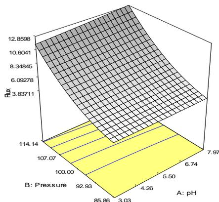
Fig. 4. Response surface plot (relationship between operating pressure, pH and permeate flux for Glucose)
