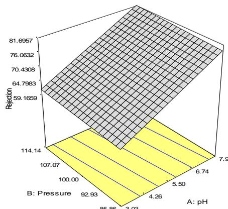
Fig. 5. Response surface plotting for the effect of controlled parameters on glucose removal efficiency
