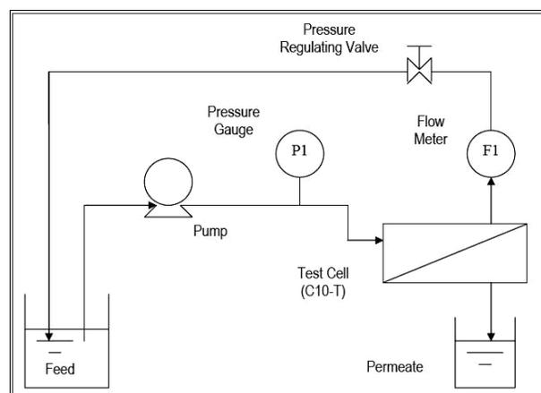
Fig. 1. LPROM set-up, Actual (left) and Schematic (right)
