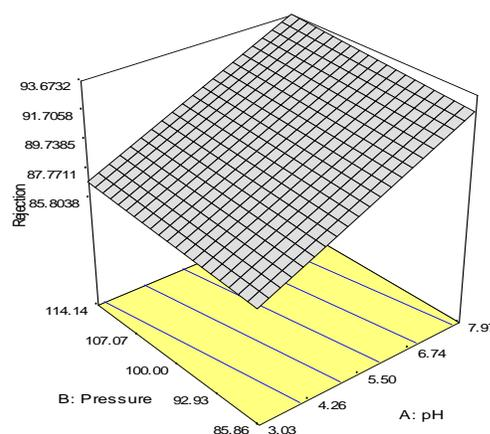
Fig: 3. Surface response plot for the effect of controlled parameters on DDT removal efficiency (relationship between operating pressure, pH and DDT removal efficiency)
