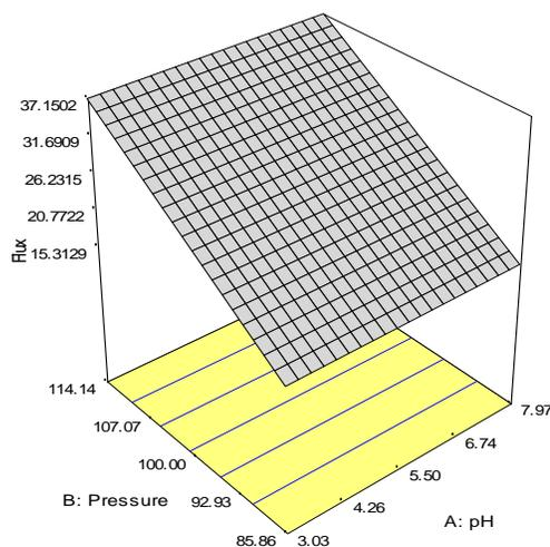
Fig: 2. Surface response plot (relationship between operating pressure, pH and permeate flux for DDT)
