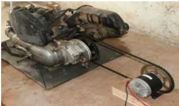
Fig. 2: Developed test bed for the hybrid vehicle
