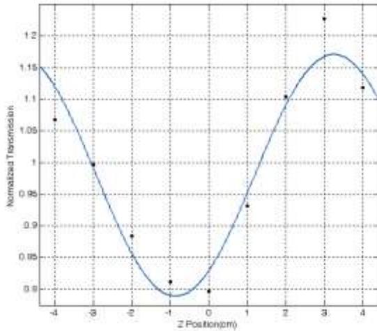
Fig. 5: Z-scan graph in the closed aperture
