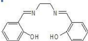
**Fig. 1:** Schiff base ligand structure (SalenH<sub>2</sub> or (N, N'-ethylenebis (salicylidene amine))
