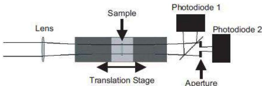
**Fig. 3:** Arrangement of Z-scan test
